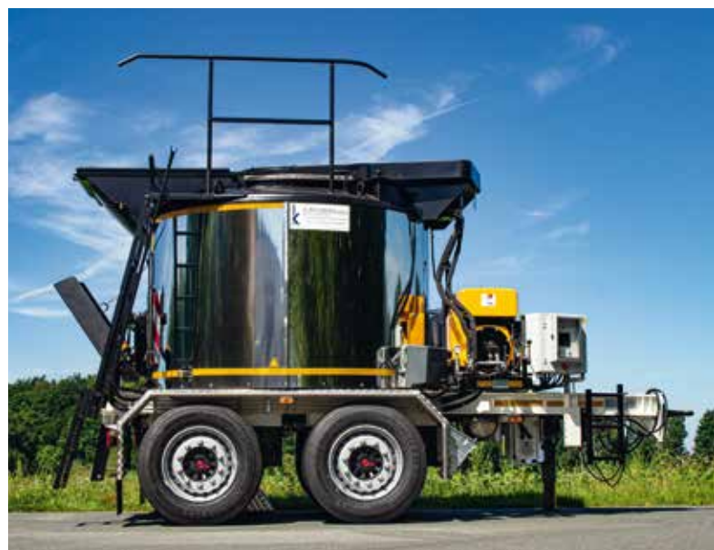
ATK H 12 boiler with high-gloss cladding and oil burner as well as other special equipment
