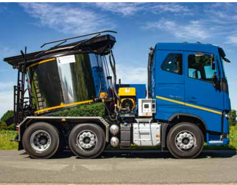
Boiler ATK H 12 with high-gloss cladding and adjustable chute on lorry and with further special equipment
