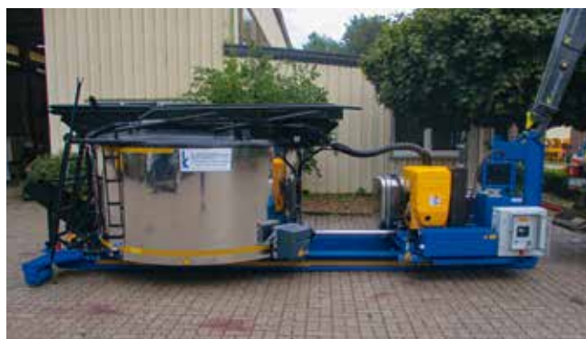
Movable boiler on roll-off frame
