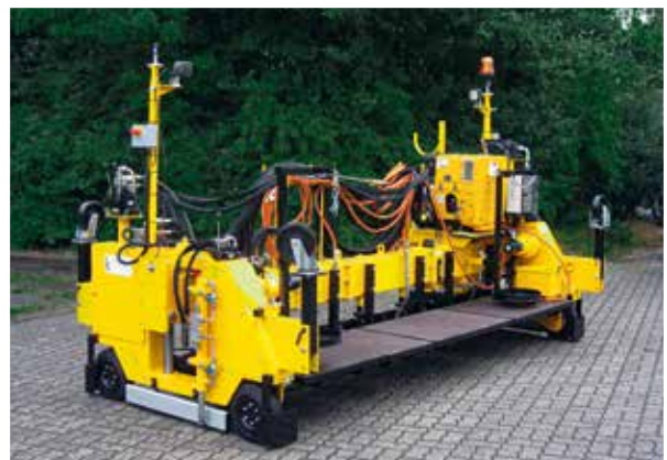
GAB 25 finisher with side strip paver and further options
