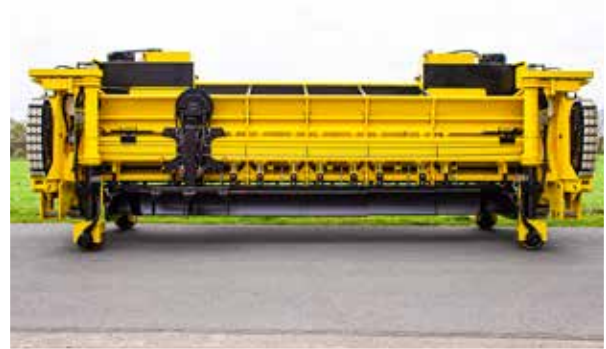
■ Mastic asphalt finisher K 110 with grit spreader and other options
