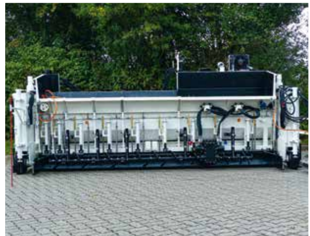
■ Mastic asphalt finisher KBR 75 SSL with blade distributor and other features
